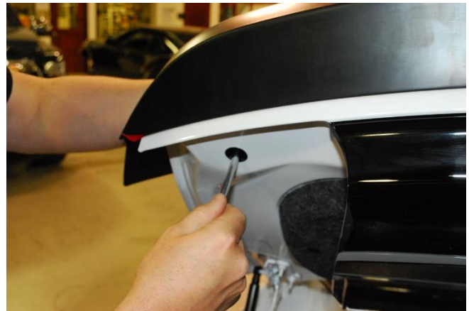
14. A.) Tighten the Spoiler Bolts. Caution: Do not over tighten. B.) Replace rubber grommets.
