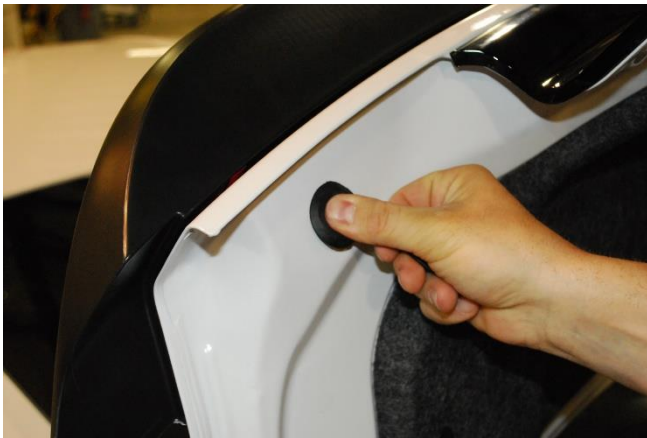
14. A.) Tighten the Spoiler Bolts. Caution: Do not over tighten. B.) Replace rubber grommets.
